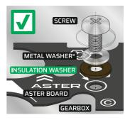
Improper placement of wiring under the motor gear may cause insulation damage and a short circuit, which is not covered by the warranty.
